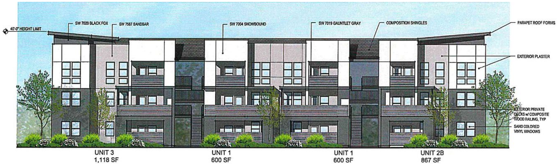
Project Elevation – Front (Building A)
